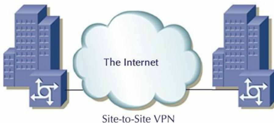
Figure 114: A site-to-site (or lan-to-lan) VPN in which the boxes with arrows represent firewalls connecting two office buildings to the Internet
