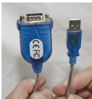
Figure 6: A USB-to-Serial adapter dongle,
